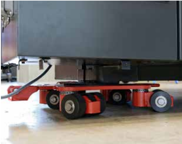
Revolving trolley JKB in action
