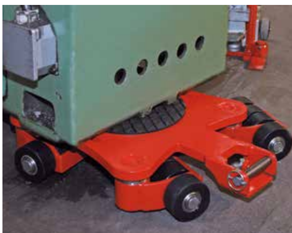
Revolving trolley JKB in action.
