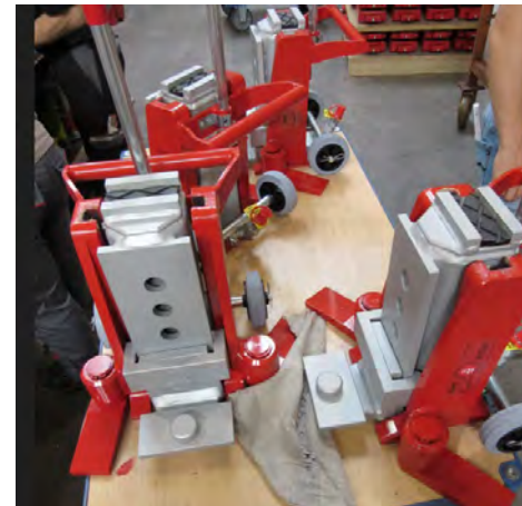
JH 15 EX with return spring, customized toe with pin and form-fitting lifting toe
