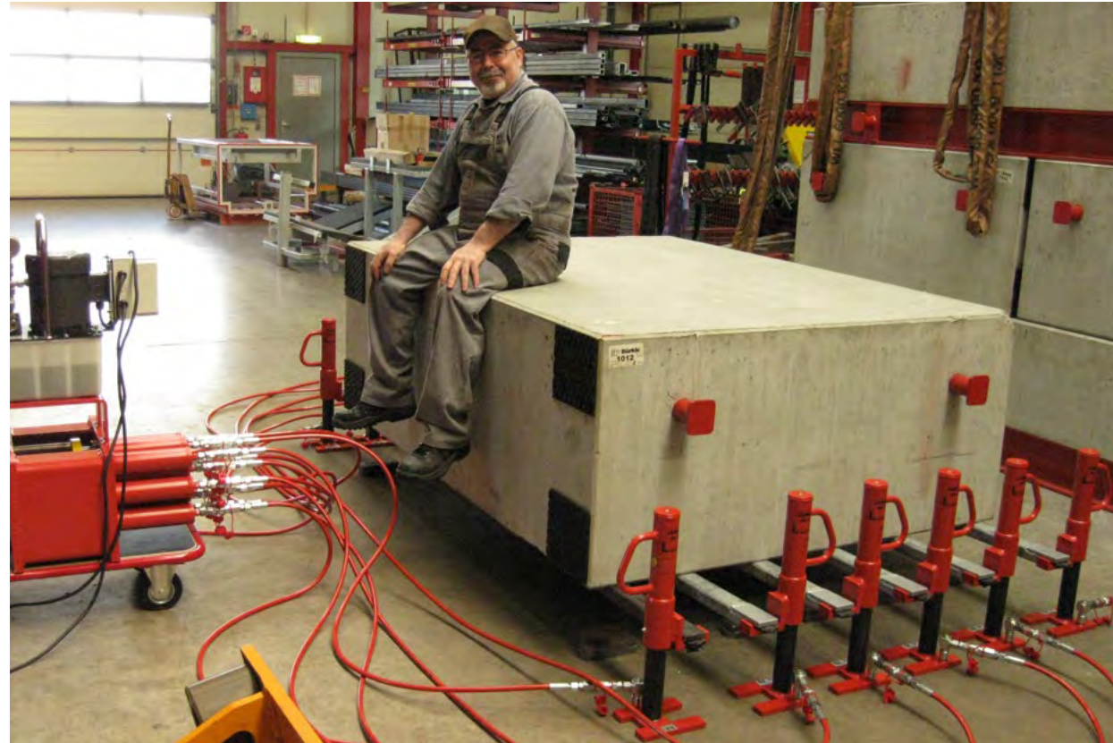
custom hydraulic pressure block with 12 ports
