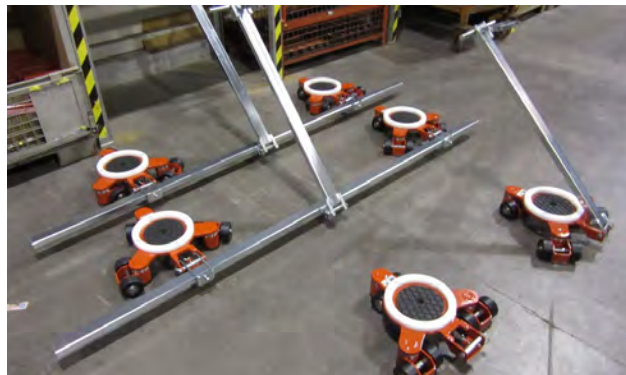
JKB 2 K with collars for machine feet und connecting bars
