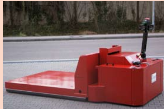
Heavy duty lift truck up to 20 tons
